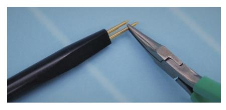
2. To fully install the new pin, position the new pin in the socket and press it against a hard surface.
