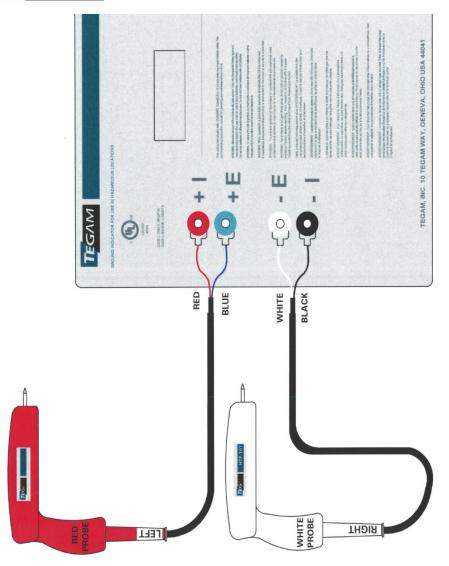
Figure 2a: HTP-101A Probe Connections
