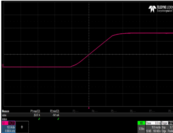
Figure 39: NP08W1-1MN0-00-A-0 Output Current Startup Characteristic Load: R = 0.55 ohm Ch 2: I_o
