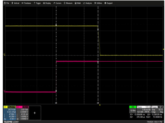
Figure 52: NP08W1-1MW0-00-A-0 Turn Off via Module Inhibit Load: I_o = 8.3A Ch 1: V_o Ch 2: Module Inhibit
