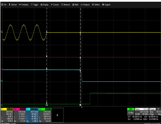
Figure 5: NP08W1-1MW0(8)-00-18P-A-0 Hold-up Time Vin = 90Vac/63Hz/0° Load: I_o = 41.67A I_{SB} = 1A Ch 1: AC Mains Ch 2: V_{SB} Ch 3: V_o Ch 4: G_PG00D
