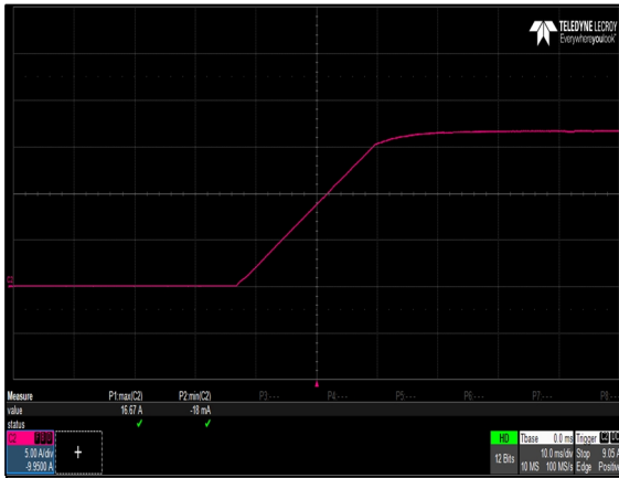
Figure 48: NP08W1-1MQ0-00-A-0 Output Current Startup Characteristic Load: R = 1.43 ohm Ch 2: I_O
