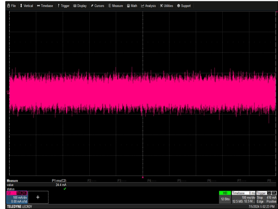
Figure 40: NP08W1-1MN0-00-A-0 Ripple and Noise Measurement Load: R = 0.55 ohm Ch 2: I_o
