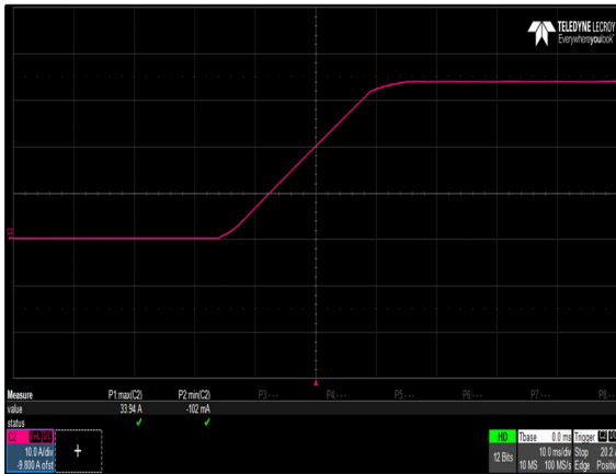
Figure 30: NP08W1-1ML0-00-A-0 Output Current Startup Characteristic Load: R = 0.36 ohm Ch 2: I_O
