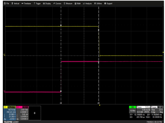
Figure 43: NP08W1-1MQ0-00-A-0 Turn Off via Module Inhibit Load: I_o = 16.6A Ch 1: V_O Ch 2: Module Inhibit
