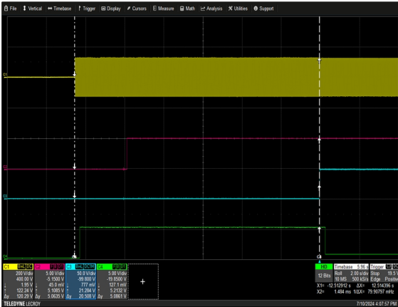
Figure 1: NP08W1-1MW0(8)-00-18P-A-0 Turn-on delay via AC mains Vin = 90Vac Load: I_o = 41.67A I_{SB} = 1A Ch 1: AC Mains Ch 2: V_{SB} Ch 3: V_o Ch 4: G_PG00D
