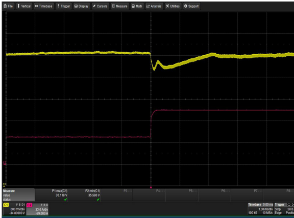
Figure 51: LCM3000U-T Transient Response - Vo Deviation 50% to 100% load change 1A/uS slew rate Vin = 230Vac Ch 1: Vo Ch 2: Io
