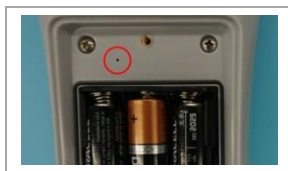
Figure 7: Alignment Access Hole Location
