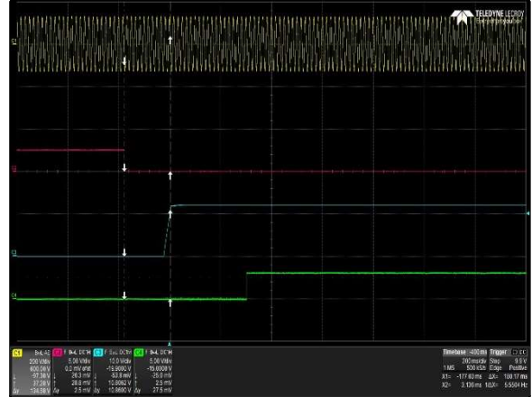
Figure 2: DS750PED-3 Turn-On Delay via PS_ON_L Vin = 90Vac Load: I O = 62.5A I SB = 3A Ch 1: AC Mains Ch 2: PS_ON_L Ch 3: V O Ch 4: Pwr_GOOD
