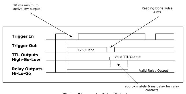
Timing Diagram for Relay Outputs
