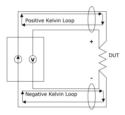
Fig 1.2: Continuity Test Paths for Broken Lead Detection
