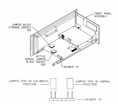
Figure: 6.1 Internal Jumpers
