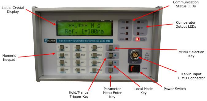
Figure 4.1: Front Panel Layout
