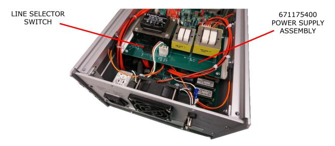
Fig 2.1: Line Voltage Selection Location
