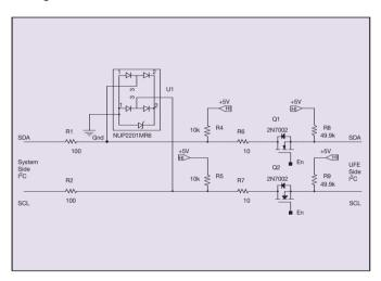
Figure 1 - Basic I<sup>2</sup>C Schematic
