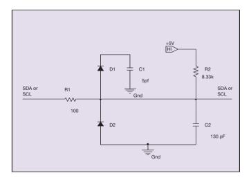
Figure 2 - Equivalent Circuit Model for the Basic I<sup>2</sup>C Schematic
