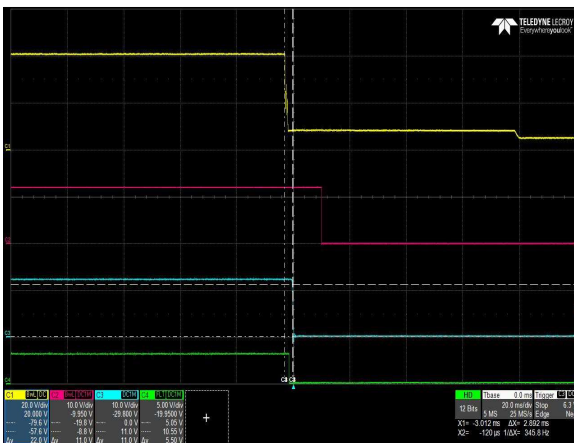
Figure 3: CSU2000ADC-3-100 Hold-Up Time Vin = -40Vdc Load: I_O = 163.9A I_{SB} = 3.5A Ch 1: V_{IN} Ch 2: V_{SB} Ch 3: V_O Ch 4: PWOK
