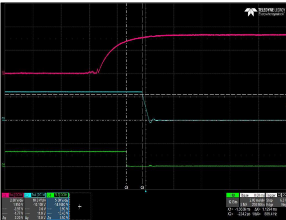
Figure 9: CSU2000ADC-3-100 Turn Off Characteristic via PS_ON Vin = -48Vdc Load: I O = 163.9A I SB = 3.5A Ch 2: PS_ON Ch 3: V O Ch 4: PWOK
