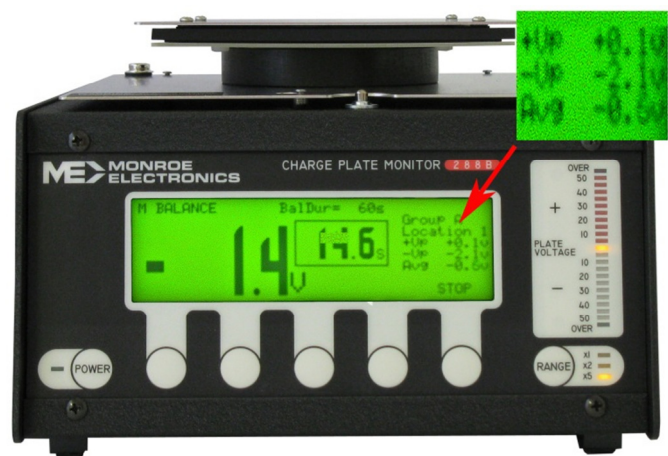
Figure 1. The Monroe 288B measuring ionizer balance.
