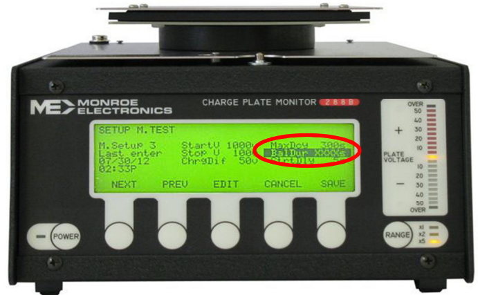
Figure 6. Selecting the balance duration to be infinite.
