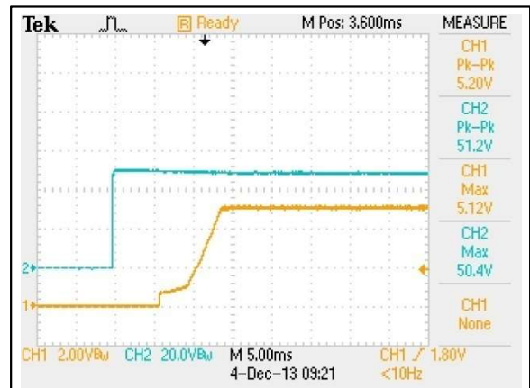
Figure 60: AEE10A36-L Output Voltage Startup Characteristic by Vin Vin = 48Vdc Load: Io = 10A Ch 1: Vo Ch 2: Vin
