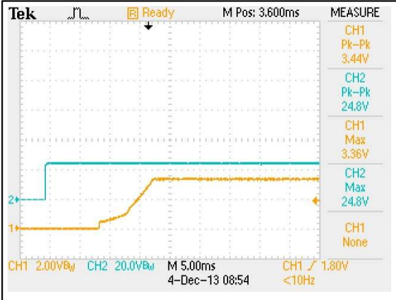
Figure 6: AEE10F18-L Output Voltage Startup Characteristic by Vin Vin = 24Vdc Load: Io = 10A Ch 1: Vo Ch 2: Vin
