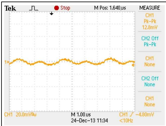
Figure 48: AEE10F36-L Ripple and Noise Measurement Vin = 24Vdc Load: Io = 10A Ch 1: Vo
