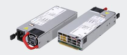
Advanced Energy's Artesyn DS2400SPE series power supply features an input range of 90 to 140 VAC, and 180 to 264VAC. It employs active power factor correction to minimize input harmonic current distortion and to ensure compliance with the international EN61000-3-2 standard - they have a power factor of 0.99 at full load. The power supplies also feature active AC inrush control, to automatically limit inrush current at turn-on to 45 A maximum.
