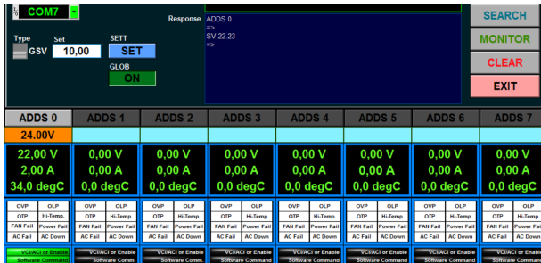
Figure 4: GUI, response to executed command “SV 22.23”
