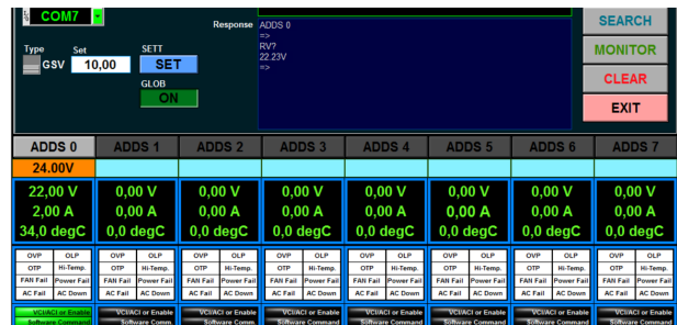
Figure 7: GUI, response to executed command “RV?”
