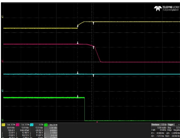
Figure 3: DS500SDC-3 Hold-up Time Vin = -36Vdc Load: I O = 41.6A I SB = 3A Ch 1: DC Mains Ch 2: V O Ch 3: V SB Ch 4: Pwr_Good
