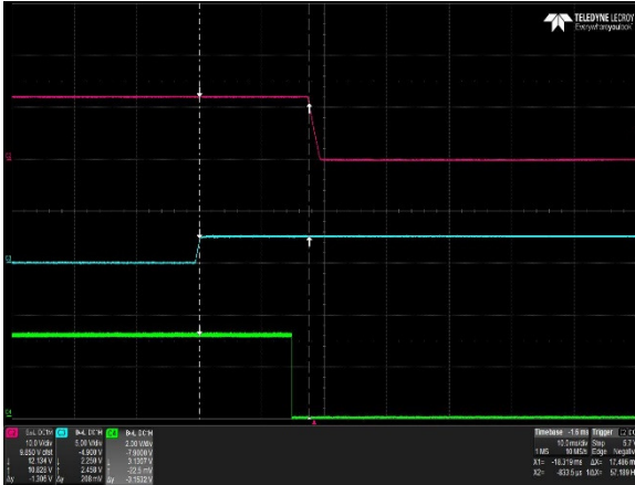
Figure 7: DS500SDC-3 Turn Off Characteristic via PS_ON Load: I_O = 41.6A I_{SB} = 3A Ch 1: V_O Ch 2: PS_ON_L Ch 3: Pwr_Good
