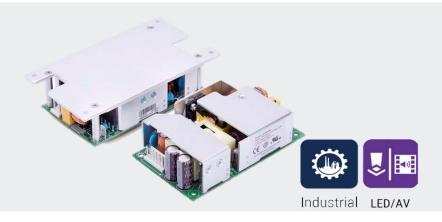
The SL Power Electronics LB240S model is the highest-density conduction-cooled power supply in a compact 3" X 5" package. Providing 240 Watts of power at 50°C ambient with 300 LFM airflow, the LB240S is designed to meet global lighting requirements and has a built-in EMI filter to meet EN55015. It has a universal AC input range of 100 to 240 VAC. All models are CE marked to low voltage directive and approved to safety standard EN60950 2<sup>nd</sup> edition and UL8750.
