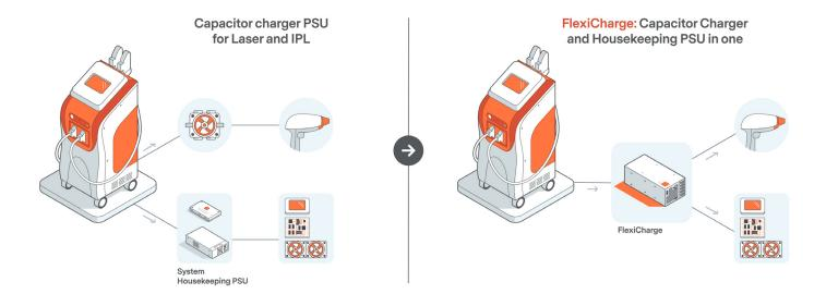
The FC1500, with its unique integrated high voltage and low voltage solution eased regulatory compliance, with reduced leakage current and simplified system EMI design. Our customer recognizes the solution and how it significantly reduced compliance time and costs while also accelerating the time to market for their system.
