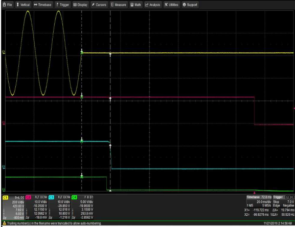
Figure 4: CSU550AP-3 Hold-up Time Vin = 264Vac/47Hz/0° Load: Io = 45A I SB = 2.5A Ch 1: AC Mains Ch 2: V SB Ch 3: V O Ch 4: PWOK
